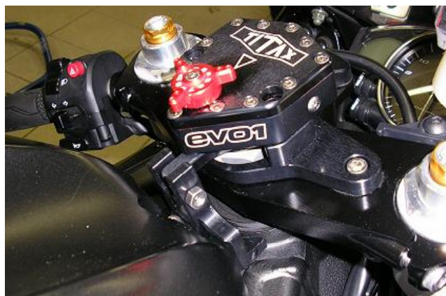
4. Screw the shock absorber with two screws M6x20 (1) to part V116/1. Secure carrier TR-04 with screw M6x35 and self-locking nut M6 (3,4).
