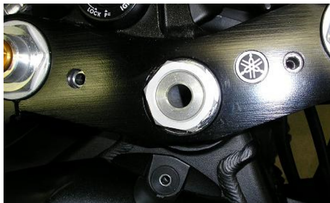
1. Dismount screws M6 on the „goggles“ and the tank.
