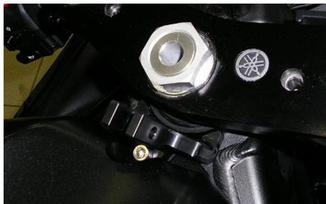
2. Mount part 133/2 on the tank under the handlebars and secure with screws (5) M6x30, (6) M5x10.
