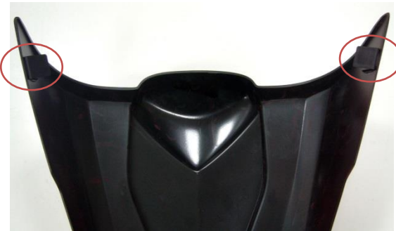
Fitting 2 : fixing brackets on sides of the seat cover
