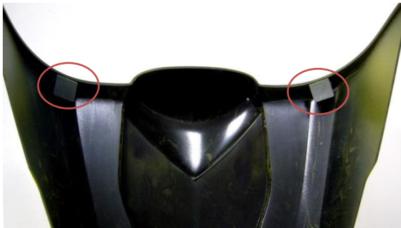
Fitting 1 : fixing brackets at front of the seat
