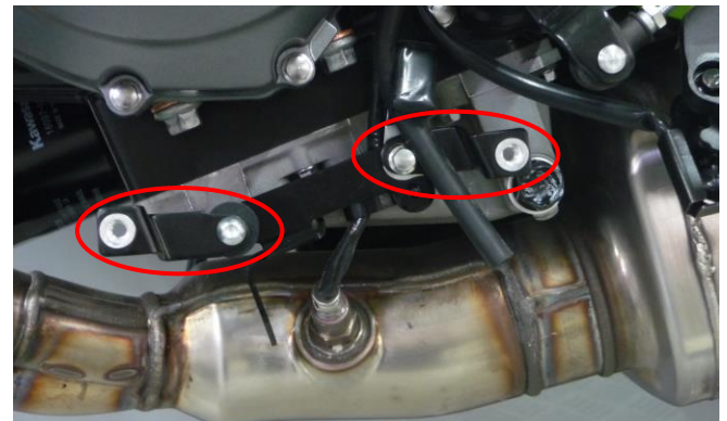
Fitting brackets on the left side
